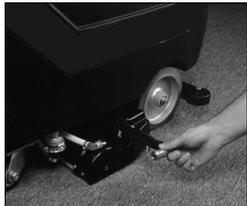
Quick disconnect spray bar slides out easily when the spray jets need to be flushed.
