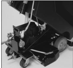
Hinged body allows access to the internal components of the machine.
