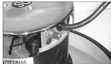
The rocker switch on the rear of the motor permits easy transition from high speed (320 RPM) to low speed (180 RPM).
