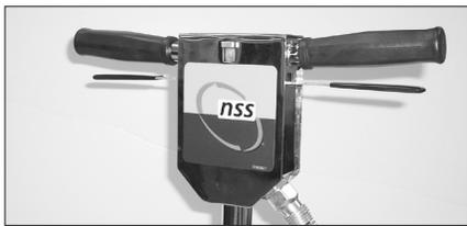
The Galaxy DS features a mechanical lock-out on the handle, which must be released before the switch lever can be activated. This important safety feature prevents unauthorized operation if the machine is left unattended.
